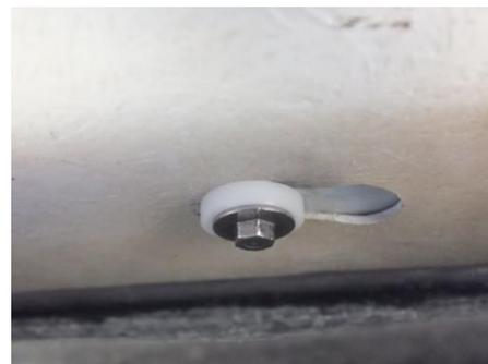
Pass the stud pin through the hole of the resinous washer. Then push up the side skirt against the body side and reinstall the stud pin to the body side together with resinous washer. As shown in the figure.
